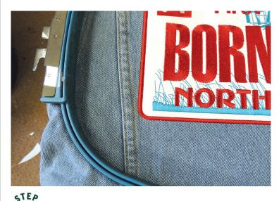
Align the design so that it doesn't sew over the seam. Attempting to sew over seams can sometimes cause stitching problems. Even if the machine sews through it, the design can appear distorted as it goes over the seam.
