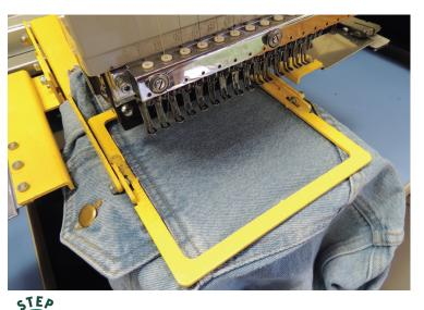
One option for hooping denim jackets are the EMS Hoop Tech bag clamps. Such clamps are particularly useful to hoop thick materials, like the front of a denim jacket.
